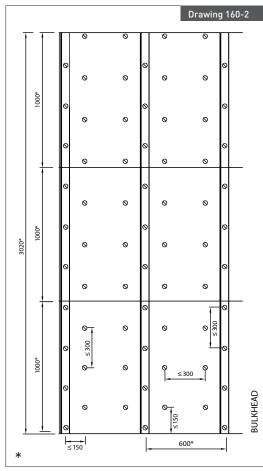
\* Dimensions may vary depending on structural design and size of insulation slab.
